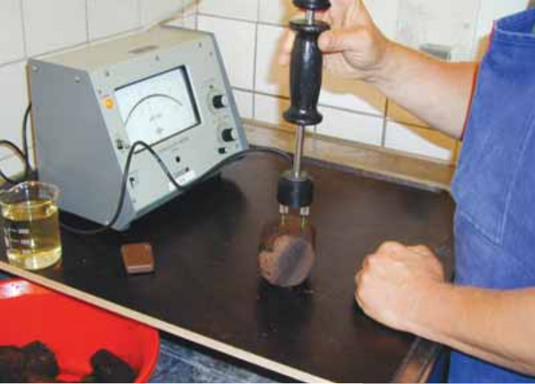
Delmhorst hand set and Radiometer (CDM3) conductivity meter showing how conductivity can be measured in samples of waterlogged archaeological wood. The use of conductivity and compression strength help to assess the state of preservation.
