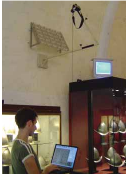
Testing of the Remote Monitoring Photo Capturing (RMPC) system, that allows to take pictures of metal coupons on a daily basis to follow the progression of the corrosion process.
